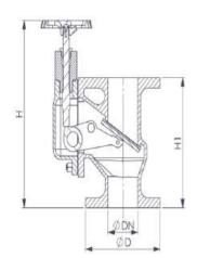
**Bronze Straight (Vertical) Storm Valve** c/w Closing Device **DIN 87101 Form B** Flanged PN16
