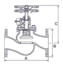
**Ductile Iron** Marine **Straight Pattern Quick Closing Globe Valve**
