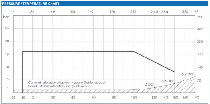
Note: This range is not suitable for steam. Do not use when the pressure & temperature are below the liquid/steam saturation line (hatched area)
