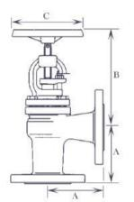
**Cast Iron Body Stainless Steel Disc Screw Down Non Return Angled Globe Valve** Flanged PN16
