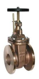
Non rising stem, metal seated gate valves, suitable for cold and hot water, seawater, saturated steam, oil and other neutral non aggressive liquids.
