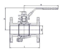
**Stainless Steel** 2 Piece Ball Valve c/w Operating Lever **Flanged PN16**
