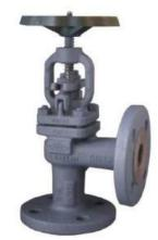
This bolted bonnet globe valve with a stainless steel valve disc has a non return design, preventing reverse flow when in the open position. Also suitable for isolation duty, providing a leak tight shut
