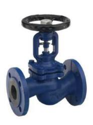
This bolted bonnet bellow sealed globe valve with a stainless steel valve disc is ideally suited for isolation duty, providing a leak tight shut off with the capability of being used partially open to regulate flow.
