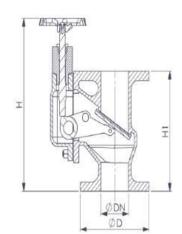
**Ductile Iron Straight (Vertical)** Storm Valve c/w Closing Device **DIN 87101 Form B** Flanged PN16
