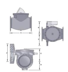
**Ductile Iron (Epoxy Coated) Body EPDM Seals** Swing Type Check (Non Return) Valve c/w Outside Lever & Weight **Flanged**
