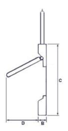
**Stainless Steel EPDM Seals Swing Type Check (Non Return) Valve Multi Flange Wafer Type** DN40 80 PN10/16/25/40. ANSI 300 DN100 150 PN10/16 DN200 400 PN16
