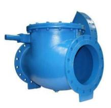
The JV080037 is a metal seated swing Approvals, Features & Benefits check (non return) valve with EPDM seals used to prevent reverse flow. In this case an outside lever and weight is fitted to the standard valve to aid closure when gravity is insufficient to close the valve fast enough.
